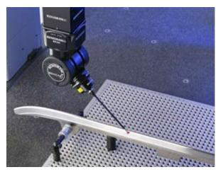
The existing blades were first sent to Renishaw's UK research facility, where its revolutionary REVO<sup>™</sup> five-axis measuring head for CMMs was used to scan the blade, quickly capturing many thousands of data points to enable its form to be defined in great detail.
