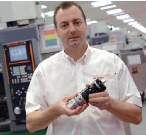
**Paul Maxted holds a probing unit, the kind used on many of the machine tools in the shop. The probe is doubly significant. Probing plays a critical role in the machining strategies established on the VMCs, lathes and turn-mills. The parts produced on these machines include most of the components for probes such as this one.**
