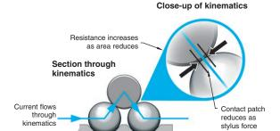
Repeatable electrical triggering and mechanical reseating of the mechanism are critical to this process and fundamental to reliable metrology.
