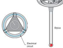
Under load of the spring, contact patches are created between the balls and the rods through which the electrical current flows. Upon making contact with (touching) a workpiece, the force translated through the stylus moves the balls and rods apart thus reducing the size of the contact patches and increasing their electrical resistance.
