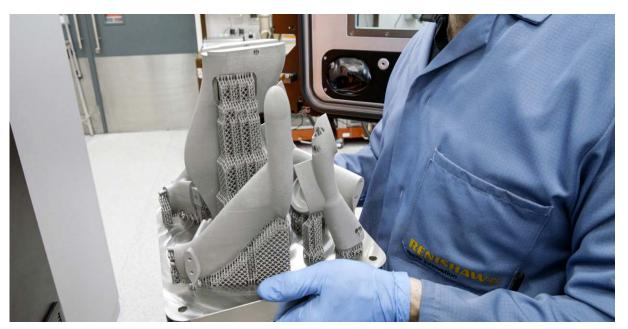
Prototype handlebar components after removal from a Renishaw RenAM 500Q additive manufacturing system
