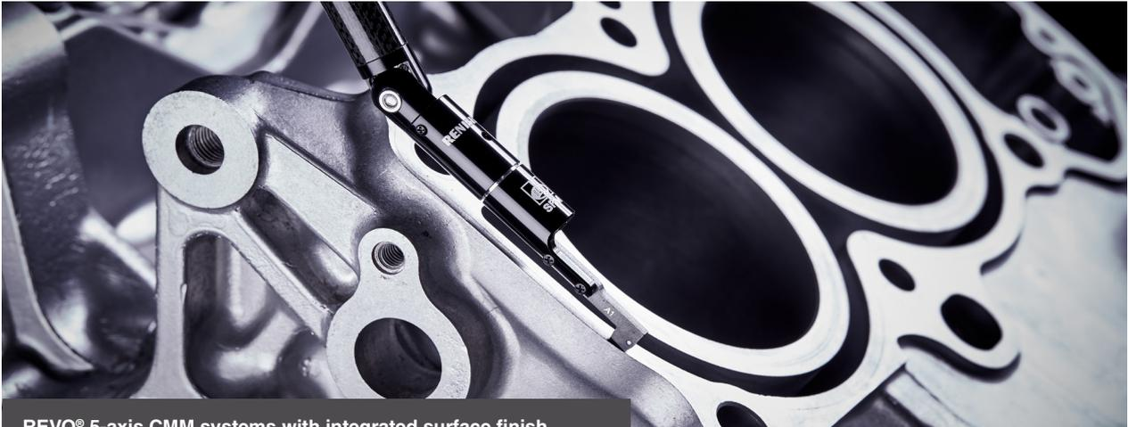
REVO® 5-axis CMM systems with integrated surface finish measurement deliver a significant improvement in inspection time and labour requirements for cylinder head quality control.
