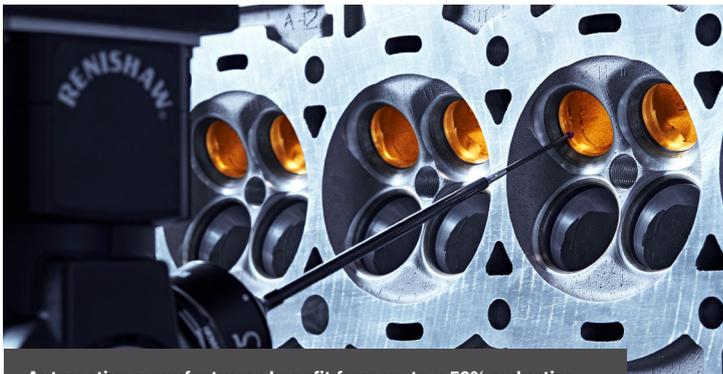
Automotive manufacturers benefit from up to a 50% reduction in cycle times when integrating surface finish measurement and dimensional inspection on a single 5-axis measuring CMM.
