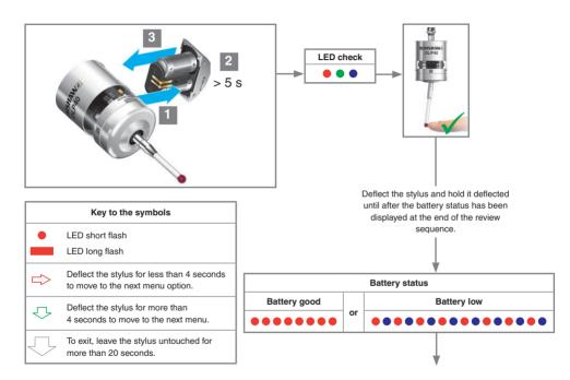
**CAUTION:** Do not remove the batteries whilst in configuration mode. To exit, leave the stylus untouched for more than 20 seconds.
