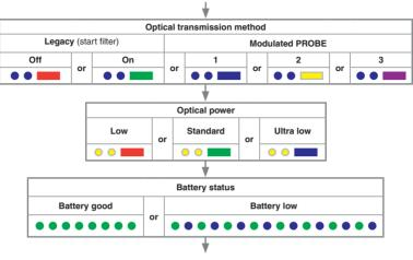
Probe in standby mode (after 8 seconds)
